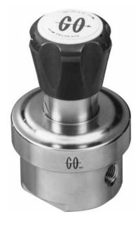
The SPR Series Subatmospheric Pressure Regulator is designed for the introduction of a low vapor pressure reactive or purge gas into a subatmospheric process The large diameter diaphragm provides optimum sensitivity for subatmospheric or positive pressure control.
