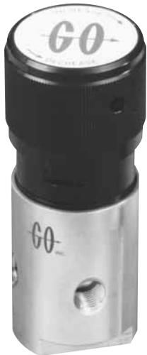
The CPR-5 Series pressure control valve is designed for service at high flows with good sensitivity and regulation utilizing a small footprint. While the design was originated for gas systems, this valve is perfectly suitable for liquid systems that are compatible with the materials of construction. Also of interest is the fact that while being able to perform with moderately high flows, this valve also provides very good performance in flow ranges of only a few liters a minute.
